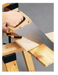
Fig. 1.6.2.9: Crosscutting with a Handsaw
