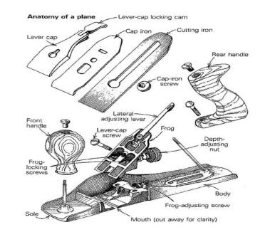
Fig.1.4.1.4: Parts of Steel Planer
