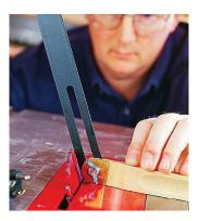
Step-3 Setting the blade angle on Table Saw
