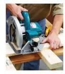
Fig. 1.6.2.7: Crosscutting With a Portable Circular Saw
