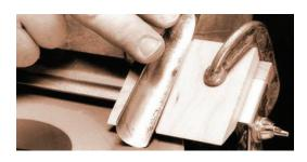
Step-2 For Sharpneing in Machine Use 'V' Groove Guide Block
