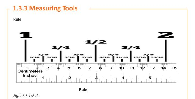
Rule is the most common and the best-known piece of measuring equipment, for measuring linear distance. Least count for Rule is normally 1 millimeter and 1/8 inch (normally one side has Centimeters and other side has inch scale).
