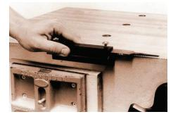
Step-1 Clamp the Saw in Saw Jointer
