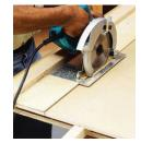
Fig. 1.6.2.5: Ripping with a Circular Saw
