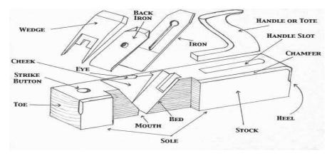
Fig. 1.4.1.3: Parts of Wooden Plane
