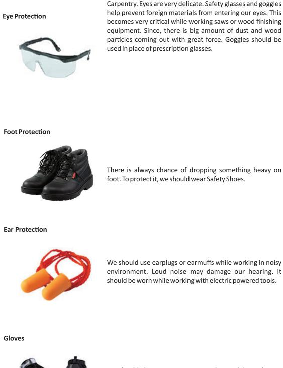
We should always use appropriate gloves while working in carpentry. There are many sharp edges we have to deal with, due to which our hand can get cut. We should use good quality cotton gloves or if required leather gloves.
