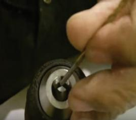
**STEP 1:** Insert the chuck key into the small hole on the side of the chuck and turn it counterclockwise until the chuck can accommodate the drill bit. Slide a bit into the chuck.
