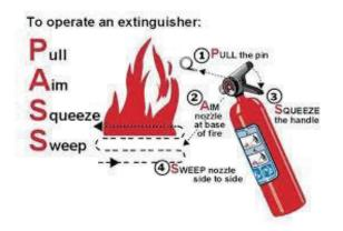
It is important that you get fire extinguisher training before you have to use one. You don't want to waste valuable time trying to read directions or figure out how to remove a pin in an emergency situation. Other important information, like how far to stand away from a fire, when to move toward it, and how long the extinguisher contents last can only be understood by actually operating one. Make sure your employer and your Safety and Health Rep know that you need this training.
