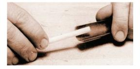
Step-5 Remove the Burr After Sharpening
