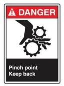
There is a threat of catching any limb by machine. Do not use the machine without Guard.
