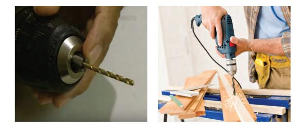
**STEP 4:** Turn on the power to the drill. Position the tip of the drill bit in the indentation, and start drilling at a low speed. Increase the speed of the drill gradually. Keep both hands on the drill as you apply pressure to the trigger. Keep the drill perpendicular to the object you are drilling to.
