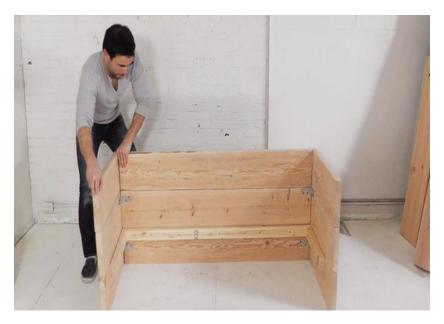
With the help of L-Brackets, wood plugs and screws, attach the base to the panel
