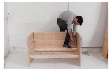
Screw the back panel to the bottom frame and the panel to the frame top
