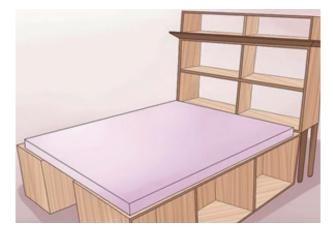
Beneath the bed frame, you can add rails and create drawers or sliding doors.
