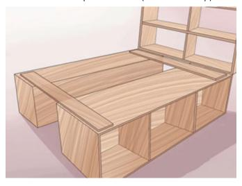
With the help of 1x10 lumber, which is cut into 16 and 3/4" you can create shelves on top of the bed frame. Secure the shelves with L Brackets (2 at one side).
