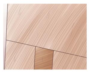
At the end shelves, add the backing. This can be done by tracing shelves onto plywood and with a jigsaw and cutting out the backing. Secure it firmly with nails.
