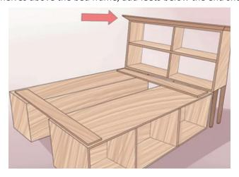
Cut 38"x75" plywood and attach at the pointed area with strong adhesive and nails.
