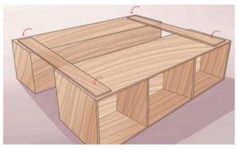
Both the ends of the two boxes will be joined with the help of two thick wood pieces of 28" 2x10. The center brace will be secured at each side with the help of L Bracket (bottom and top).
