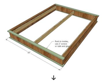
With the help of nails and glue, attach all the gaps. This will reduce the gap between the bed and the mattress space.
