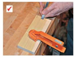
Fig. 4.1.6.1: Proper Technique of Working with Hand Tools (Use Clamps)
