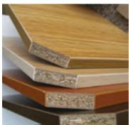
Fig. 2.3.2.9: Samples Of Particle Board (Chipboard)
