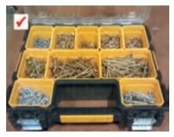
Fig 10.1.6: Always keep the sharp objects like nails, screws at the allotted box; don't leave them scattered
