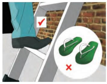
Fig 9.2.2.7: Wear safe boots, don't wear sandals or slippers
