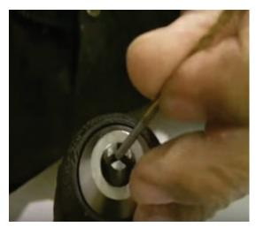
**STEP 1:** Insert the chuck key into the small hole on the side of the chuck and turn it counterclockwise until the chuck can accommodate the drill bit. Slide a bit into the chuck.
