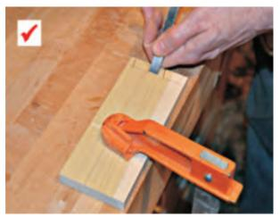
Fig 9.2.2.4: Proper technique of working with hand tools (use clamps)
