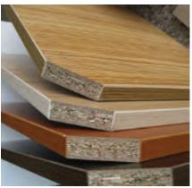
Fig 3.2.1.8: Samples of particle board (chipboard)
