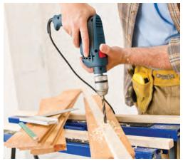
**STEP 4:** Turn on the power to the drill. Position the tip of the drill bit in the indentation, and start drilling at a low speed. Increase the speed of the drill gradually. Keep both hands on the drill as you apply pressure to the trigger. Keep the drill perpendicular to the object you are drilling to.
