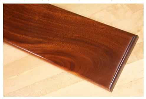
Fig. 1.5.16: Finish using Dye Stain
