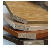
Fig. 1.3.10: Samples of particle board (chipboard)
