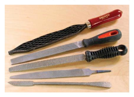
Fig. 1.5.18: Files and Rasps for Woodworking
