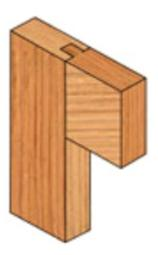
Fig. 1.4.84: Assembled Haunch Mortise and Tenon Joint
