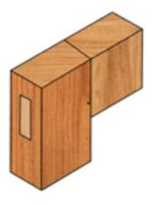
Fig. 1.4.80: Assembled Through Mortise and Tenon Joints
