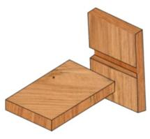
Fig. 1.4.86: Full Housing Joint
