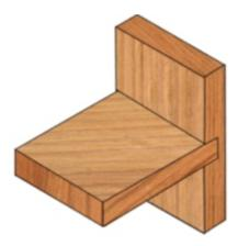
Fig. 1.4.87: Stopped Housing Joint
