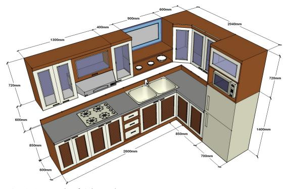
Fig. 1.2.10: Layout Plan of Kitchen Work zones
