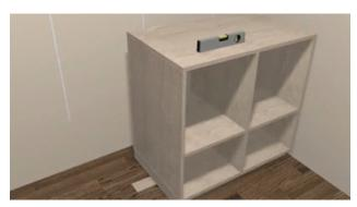
Fig. 1.4.41: Shimming the surfaces
