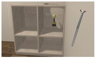
Fig. 1.4.42: Fixing the lower cabinet to the wahll
