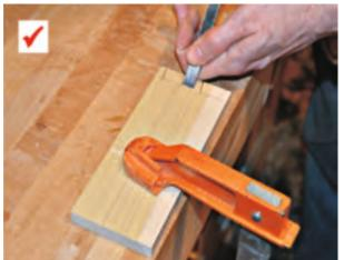
Fig 9.2.2.4: Proper technique of working with hand tools (use clamps)
