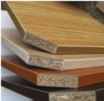
Fig 3.2.1.8: Samples of particle board (chipboard)
