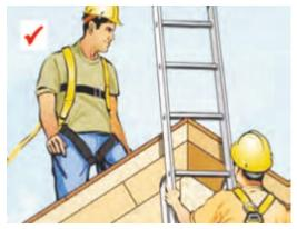
Fig 9.2.2.1: Correct posture of working (always wear safety jackets)
