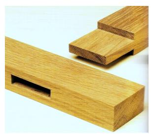
Fig 3.1.6.1: Mortise and Tenon Joint
