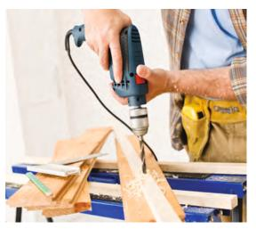
**STEP 4:** Turn on the power to the drill. Position the tip of the drill bit in the indentation, and start drilling at a low speed. Increase the speed of the drill gradually. Keep both hands on the drill as you apply pressure to the trigger. Keep the drill perpendicular to the object you are drilling to.
