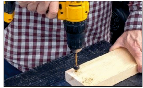
Fig 24: Pilot Holes for Screws
