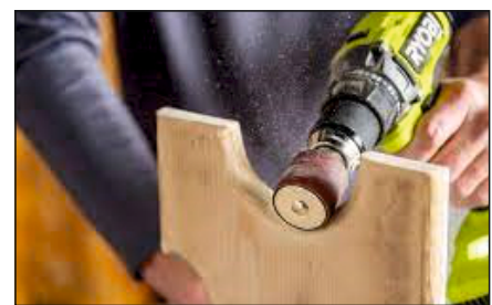
Fig 25: Sanding with Drill Attachment
