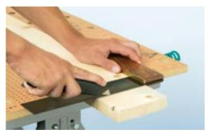
**STEP 3:** Score along the guide line using a utility knife.
