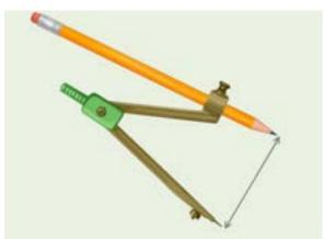
**STEP 2:** Adjust the angle of the arms so that they span the full desired radius.
