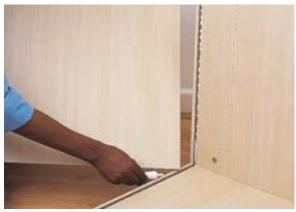
STEP 9: Secure the first side panel by tightening the two cam nuts. Use a screwdriver to turn them clockwise.
