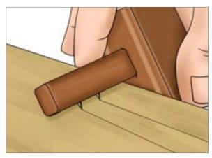
**STEP 3:** Curl your hand around the fence and tilt it slightly in the direction you are going to mark. Then simply drag the fence along the workpiece, applying very little pressure.
