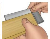
**STEP 6:** Assemble all three pieces together using bridle joint and check.
