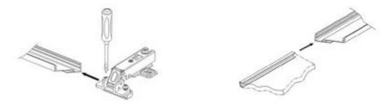
**STEP 3:** Insert the hinges in the track and tight the screws properly.
