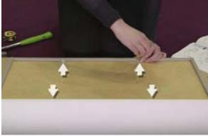
**STEP 11:** Take the wedges and slide the flange into the groove. Tighten the screw clockwise using a screwdriver. Repeat the process for the remaining wedges.
