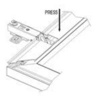
**STEP 5:** Insert the glass panel in the track and join the aluminium profiles with corner connectors.
