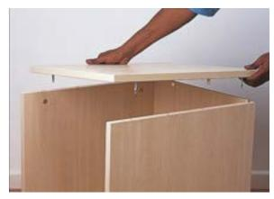
STEP 11: Slide the second side panel into position and tighten both the cam nuts.
