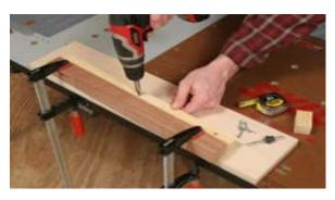
STEP 3: Cut a straight, flat piece of scrap to make the support the same length as the leg. Set the support against the leg, and fasten it to the base with a few countersunk wood screws.
