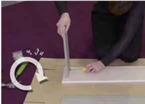
**STEP 5:** Now, take a side panel and line up with the hole of front panel. Push the side panel onto the front until it is flush. Tighten the cam barrel clockwise with a screwdriver, ensuring it is locked in place.
