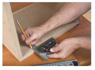
STEP 9: Set the gauge at 7/8 inch offset (1/8 inch setback  $+ \frac{3}{4}$  inch drawer face) and mark a line along with the side edge of the carcass.
