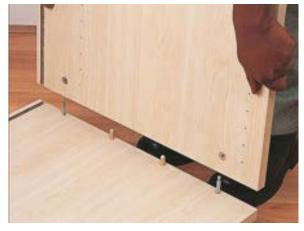
STEP 7: Now, put a dab of PVA wood adhesive on the end of each dowel that's sticking out.
