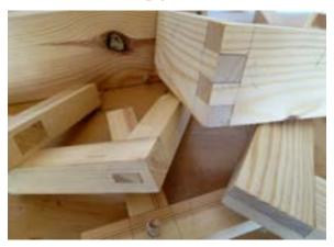
Woodworking joints is the spot where two or more pieces of wood are joined together to form a structure. Each joint has its own strength and appearance. That is why different types of joint are used for different purpose. Adhesive, glue, or fasteners such as nails, screws, bolts are used to increase the strength.
