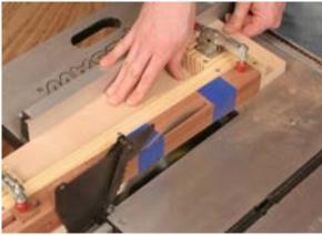
STEP 8: To taper the other face, tape the cutoff piece back in place, and flip the leg in the jig so the offcut face is up. Adjust the clamp bumpers and clamp the piece, and make the second taper cut.
