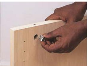
**STEP 5:** Tap the dowels into place with a small hammer (they should fit snugly). Take care not to damage the end of the dowels; a light tap should do the trick.
