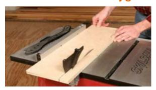
STEP 1: Make a base for the jig from 3/4 inch plywood. Rip and crosscut the base to size so it is at least 6 inch wide and about 6 to 8 inches longer than the leg you want to taper.
