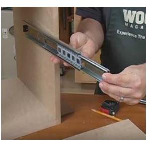
**STEP 1:** Before you mount the drawer slides you need to separate them, so that one part can be mounted onto the side of the carcass and the other onto the drawer. There is no right or left unit, so select either unit to begin. To separate the slide, press down the black plastic release lever on the inside of the smallest section of the slide, and pull until this small section separates from the unit. This small section is the drawer member. The large section is the cabinet member.
