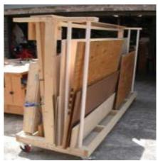
Fig: Ways of Storing Cut Sheets
