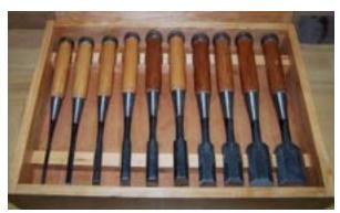
Fig: Storage of Chisels in a Chisel Box
