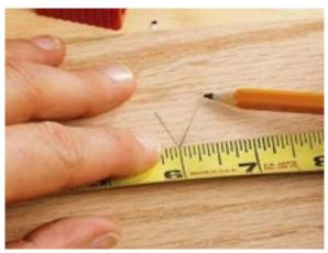
STEP 4: Mark the length by drawing an arrow with the pencil.
