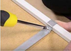
**STEP 12:** If the drawer is too wide, use metal brace under the drawer back. Take the metal drawer box brace. Note that there are two fixings required. Hook the brace over the drawer back and position it at centre. Fix the brace at the back and front of the drawer box. Now, the drawer box is ready!
