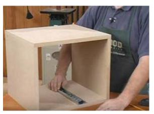
STEP 7: Set the other drawer member against this piece of wood. Set the 1/8 inch offset from the front of the drawer. Fasten the drawer member with the screws.
