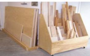
Fig: Storing small offcut plywood pieces in open boxes
