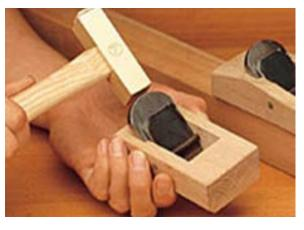
**STEP 2:** Adjust the angle of the blade with the help of mallet.
