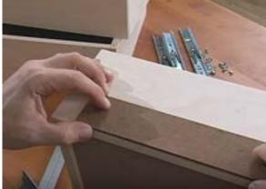
**STEP 5:** Now, take a piece of scrap wood and place it below the mounted drawer member. Mark a point on it where the bottom of the drawer meets and cut it.
