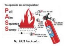
Pull the pin at the top of the extinguisher. The pin releases a locking mechanism, allowing you to discharge the extinguisher.
