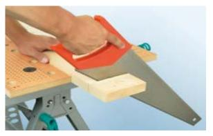
**STEP 7:** Begin to saw through the wood, back and forth, using long strokes.
