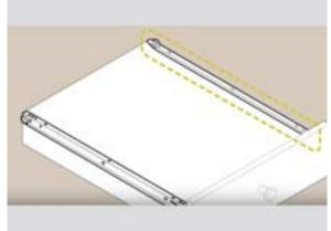
**STEP 3:** Keeping the drawer front on your right, place the drawer upside down. Take the slide that is marked 'DR'. Now, position the slide 'DR' such that the wheel is at the back with the front of the slide tight against the back of the drawer front. Secure the slide 'DR' to the base of the drawer using a screwdriver and screws provided.
