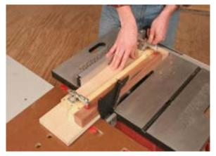
**STEP 7:** Start the saw, and feed the jig along the fence to rip the taper. Keep your hands behind the jig support throughout the cut.
