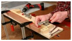
step 5: Make two mounting blocks for the toggle clamps from scrap the same thickness as the leg. Fasten the blocks behind the support and near the ends of the leg.
