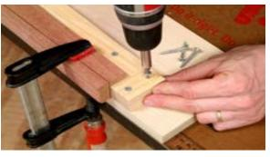
**STEP 4:** Attach a stop block to the jig that butts against the end of the leg. Fasten it with a couple of screws.
