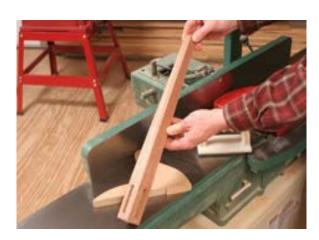
STEP 9: Now run the tapered faces over the jointer to remove the blade marks, and scrape or sand them smooth.
