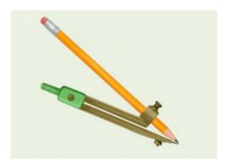
**STEP 1:** Secure a sharp pencil in the clamp of a compass. Align the pencil lead with the compass's needle.
