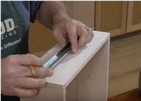
STEP 2: Using try square and pencil, draw a centerline on the center of drawer side.
