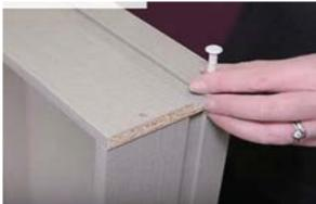
STEP 9: Ensure the holes of back panel and side panels are aligned. Carefully drive the screw or plastic nail into the holes. Turnover the drawer box and repeat the process with the other side.
