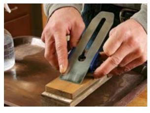
**STEP 1:** Sharpen the blade of plane on oilstone.
